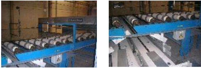
Figures 69 And 70: Glass On Roller Bed Production Line Being Scanned For Impurities
