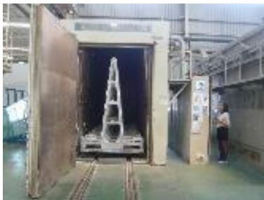
Figure 78: “A”- Frame On Roller Track Where Glass Sheets Are Placed During Heat Soak Process Inside The Heat Soak Oven (Courtesy: AgFacadesign & G Facadesign Pte Ltd)
