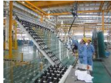
Figures 82, 83 And 84: Glass Coming Out Of Cleanroom And The Heat Machine And Lifted Off
