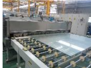
Figures 82, 83 And 84: Glass Coming Out Of Cleanroom And The Heat Machine And Lifted Off
