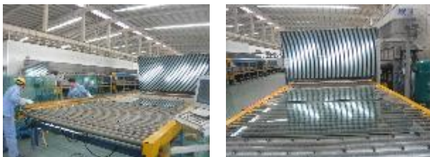
Figures 76 And 77: “Zebra Board” Lines Reflected For Visual Check On The Processed Glass Flatness At End Of Tempering Process (Courtesy: AgFacadesign & G Facadesign Pte Ltd)
