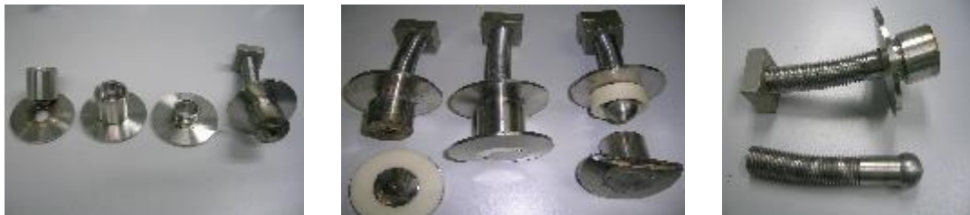
Figures 171, 172 And 173: Material Testing Of Bolts
