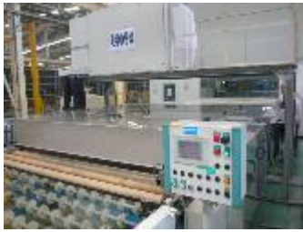
Figures 79, 80 And 81: Glass Is Cleaned Before Entering The Cleanroom Where PVB Sheet Is Laid
