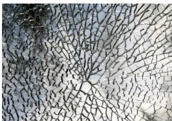
Figure 88: Tempered Glass (Courtesy: Pixabay.com)
