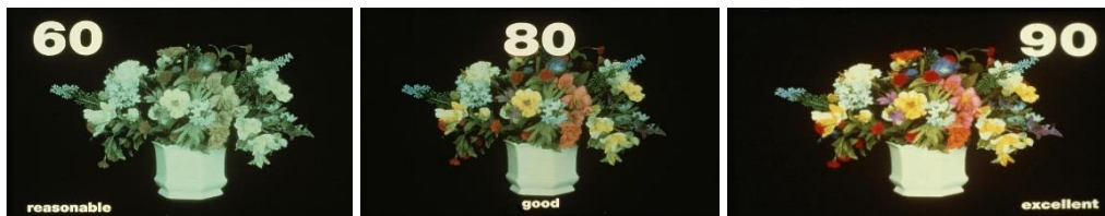
Figure. 244. Different CRI At Same Lighting Level
