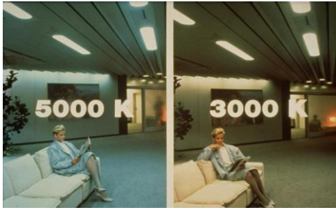
Figure 241 Illustration Of Colour Temperatures In An Interior (Image Credit: Philips Lighting)
