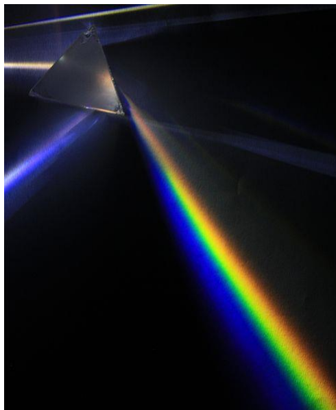
Figure 198: Separation Of Light By A Prism According To Wavelength (Image Credit: D-Kuru/Wikipedia Commons)
